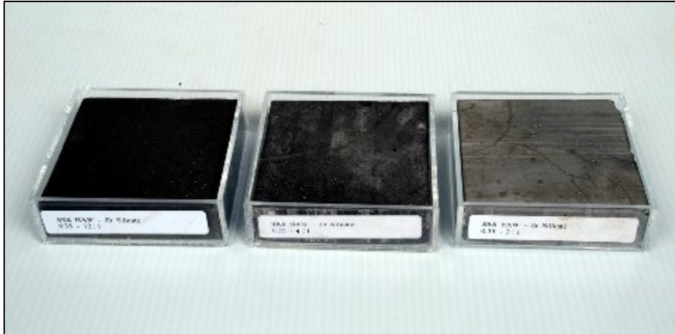
Fig. 2. Zirconium silicate samples at the W/C ratio of 0.35.
