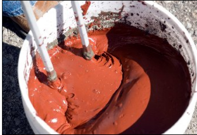
Fig. 4. Iron oxide sample after mixing.
