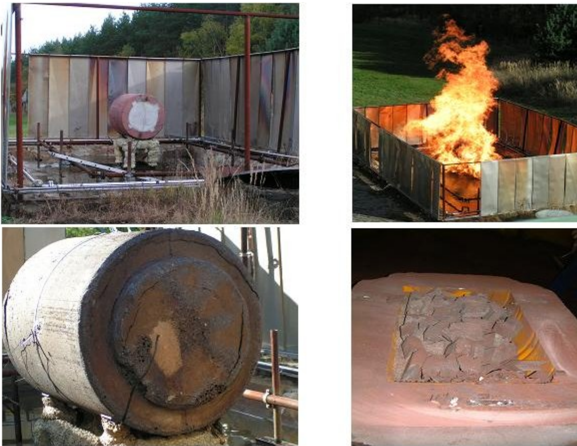
Fig. 3. Concrete container Konrad Type I fire test; ABK I+II with accident safe waste packaging. The figures above show the experimental set-up before and during the fire test. The figures below illustrate the container after the test (general and cross-section view).
