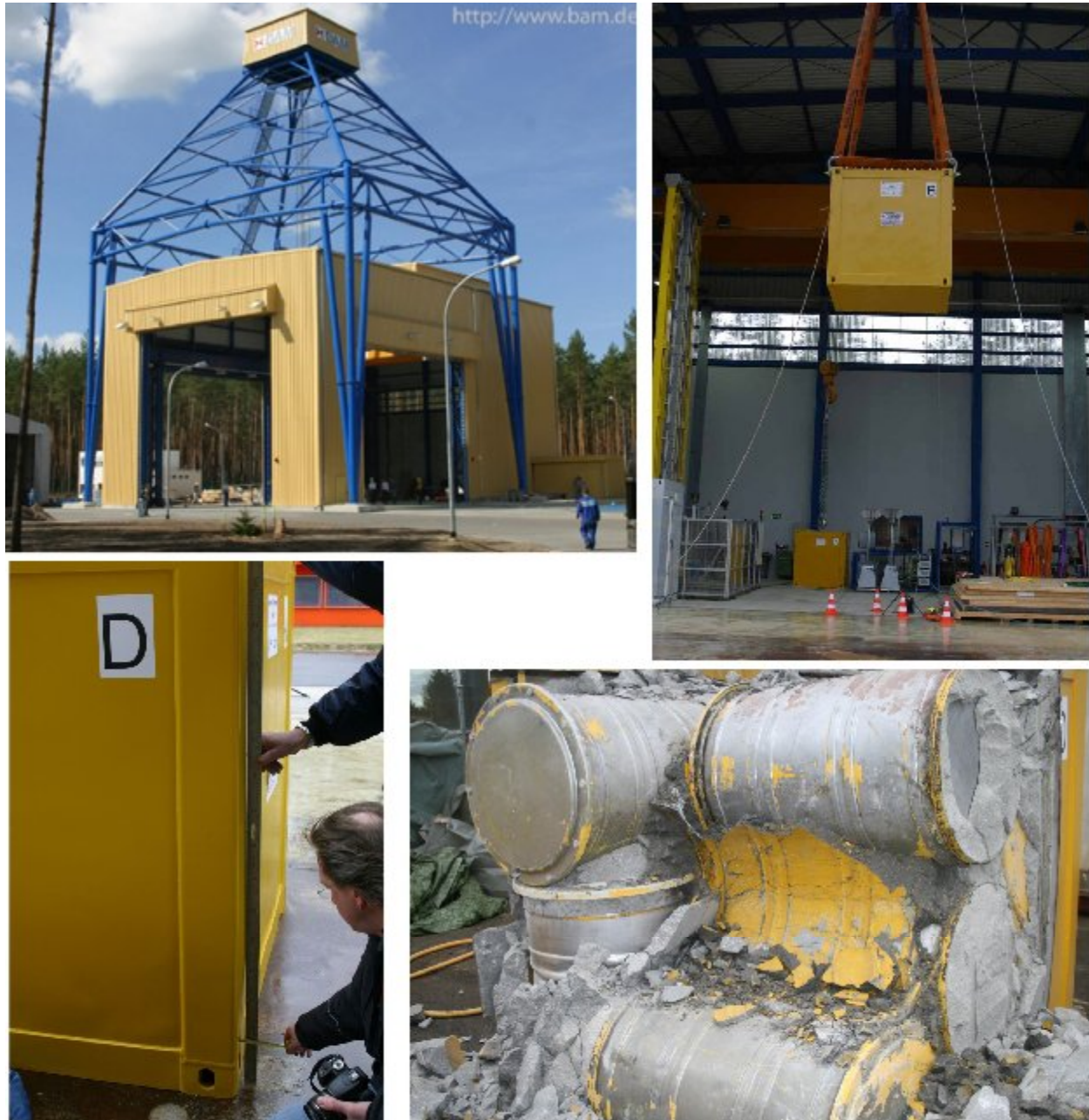
Fig. 2. 5 m drop test of a steel container Konrad Type II (ABK I with accident safe packaging) manufactured by Eisenwerk Bassum GmbH at the BAM drop test facility. Left bottom picture shows minor plastic deformation without loss of integrity after the test. Right bottom picture shows investigation of 200 liter drum condition.
