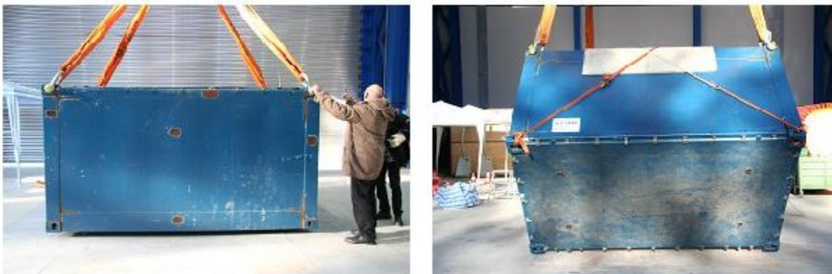
Fig. 4. Steel container Konrad Type V (old) including 26 charged 200 liter drums fixed with concrete; ABK I; drop test: 80 cm height.
