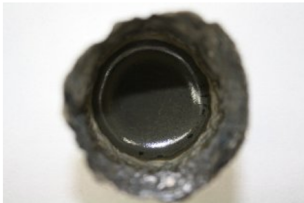
Fig. 4 Photograph of a phase segregated glass after heat treatment
