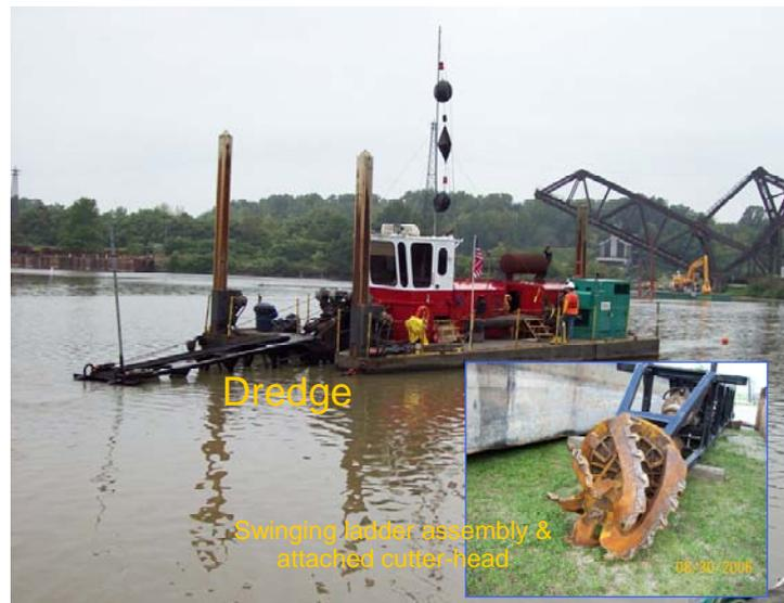
**Fig. 3 Dredge and swinging ladder assembly with attached cutter-head (insert).**
