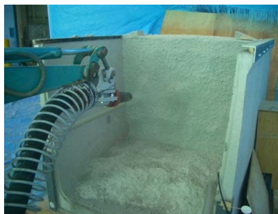
Photo 2 Full scale shotclay construction experiment
