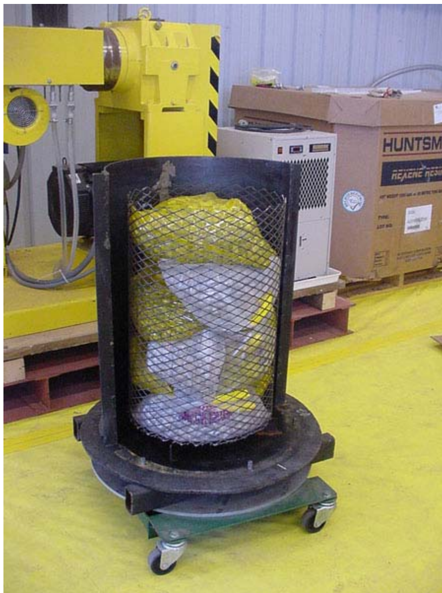
Fig. 3 Waste spark gap tubes ready for macroencapsulation at SNL
