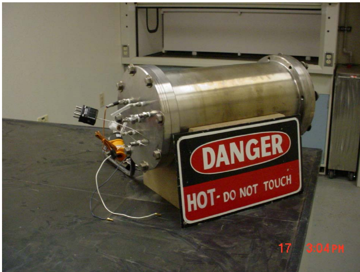
Fig. 2 SNL “boom box” used to inert explosively reactive mixed wastes and materials
