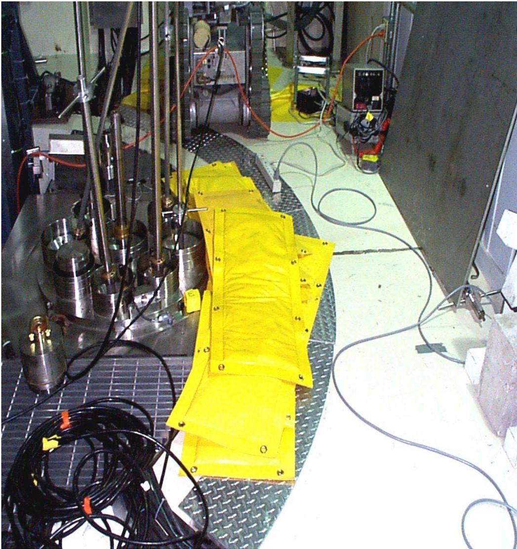
Fig. 4. Lead Blankets over the Source.
