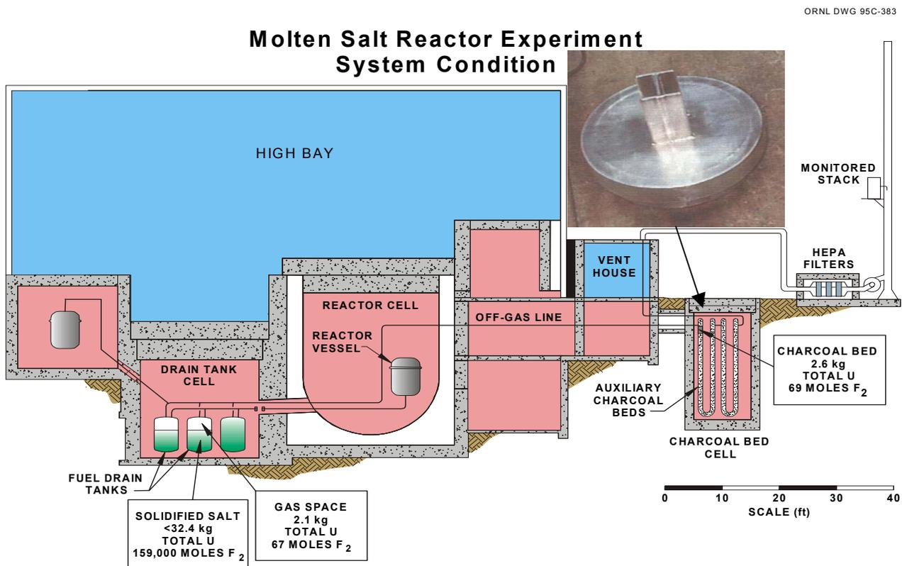
Fig. 3. Diagram of MSRE design<sup>b</sup>, with an inset photographic enlargement of lead-cap shield.
