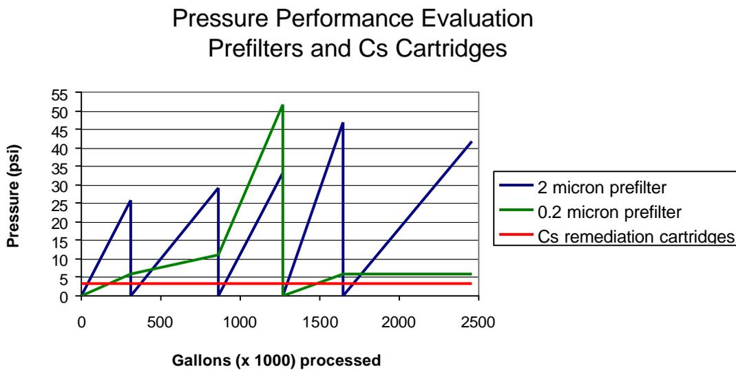
Fig. 3. 3M SRS R-Basin Pressure Performance
