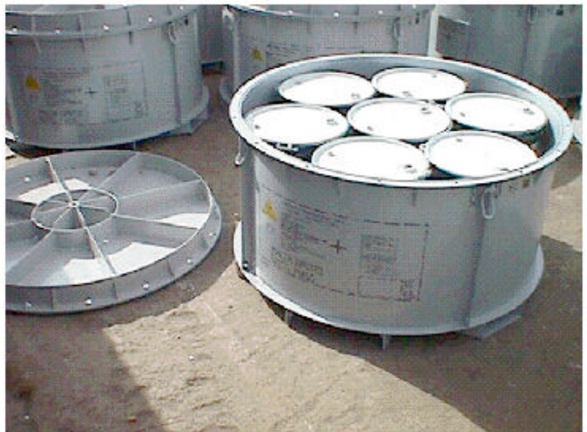
Fig. 3 The new SRW transport and storage container by forklift, from both sides of the container.
