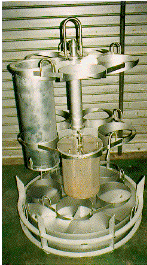
Fig. 3: The special structure for the transportation of the strainers filled with swarfs. The picture shows also a filter cask for the transportation of high radiating fine filters.
