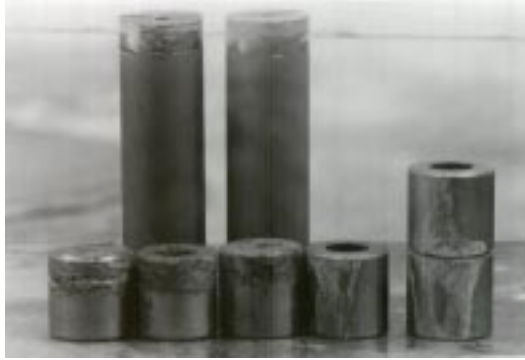
Figure 4: Compacts and Fuel Boxes with Witness Markings Resulting from Corrosion of Mild Steel Tubes
