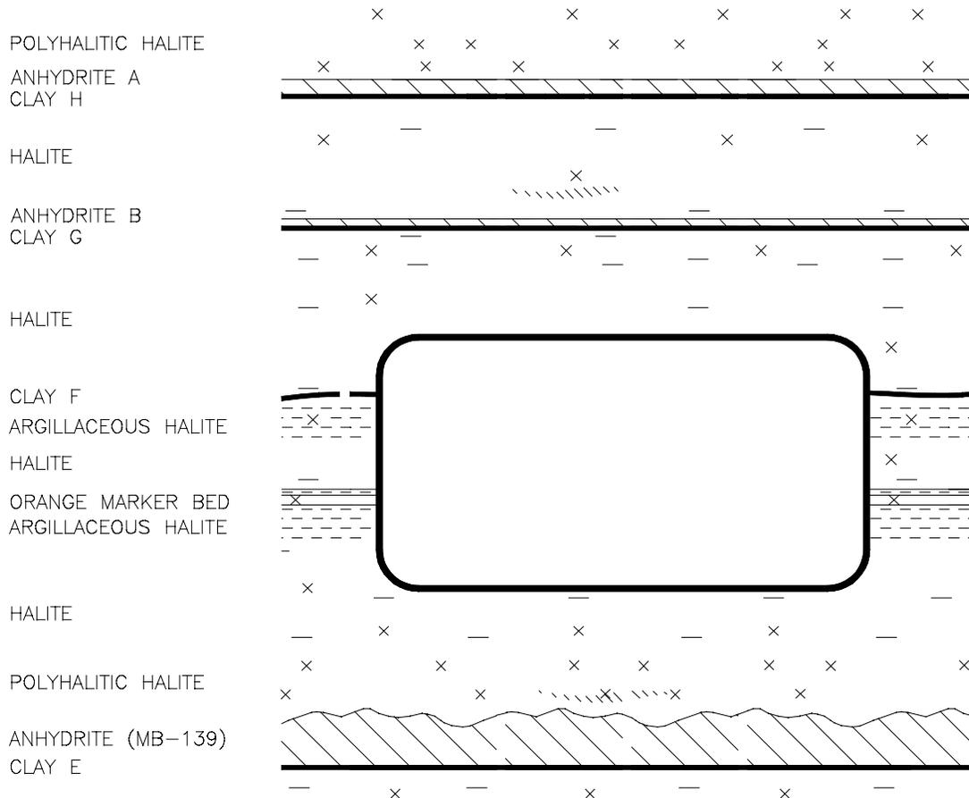
Fig. 2. Typical Geologic Cross-section.
