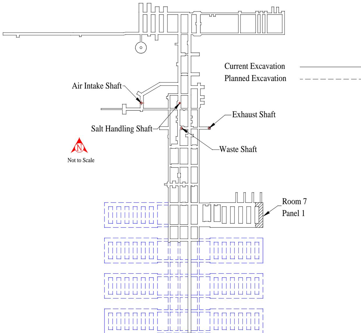
Fig. 1. Plan View of the WIPP Underground Facility
