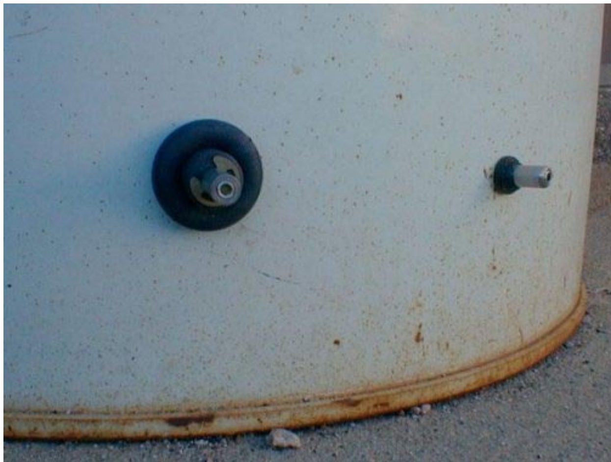
Fig. 2. Model B1, right, and Model B2, left, after being left behind in the wall of a 55-gallon drum filled with water. Once in place, multiple samples can be taken through each tool.
