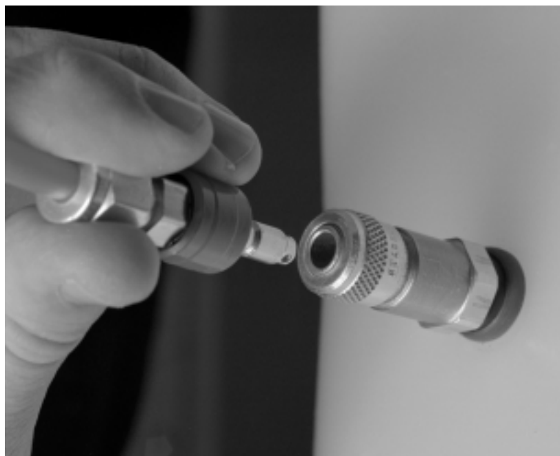
Fig. 3. Model B1-QC consists of a Model B1 modified to contain a commercial Quick Connect female connector. This makes it possible to quickly attach plumbing, valves, an alarm, or other instrumentation.
