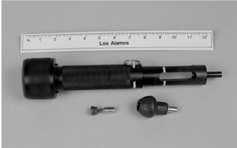
Fig. 1. Sealed-Container Sampling Tools—Model A (top), Model B1 (bottom left), and Model B2 (bottom right).
