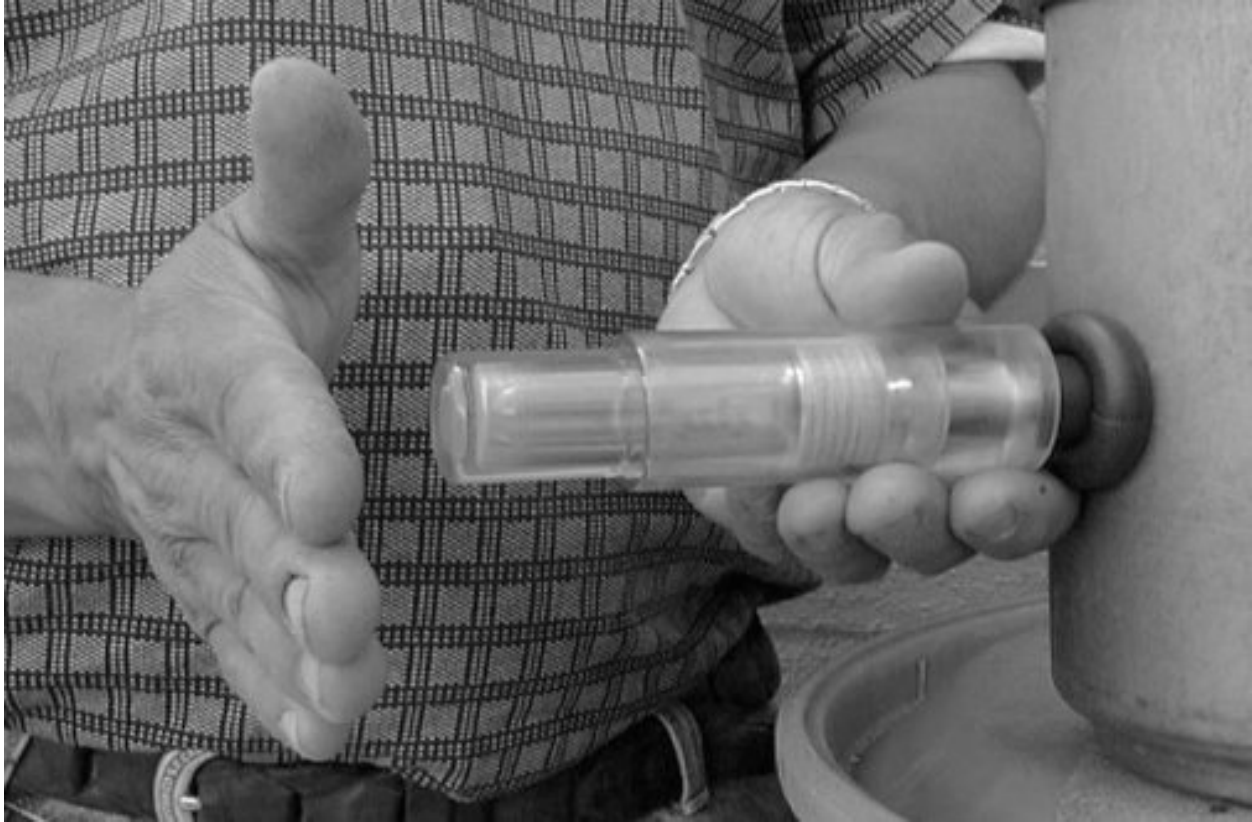
Fig. 4. Sampling with Model B2. The user pushes the clear, polycarbonate Sampler containing a Vacutainer onto the Model B2 (or B1) drill assembly and gives the back of the Sampler a shove.
